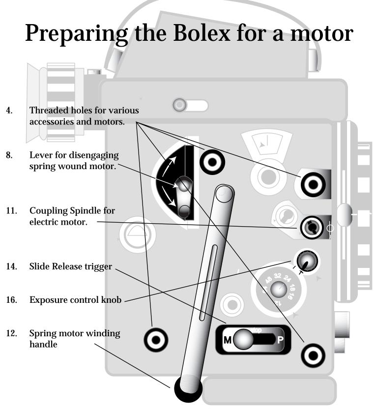
These are all the features that you have to worry about when you mount a motor onto the Bolex. The spring motor wind handle(#12) has to be removed by rotating it clockwise.
